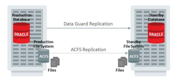
Figure 1: Data Guard and ACFS Replication
