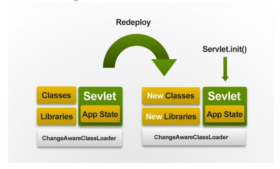
Calling Servlet.init() recreates the "initialized" application state with the updated classes loaded using the new classloader instance.
