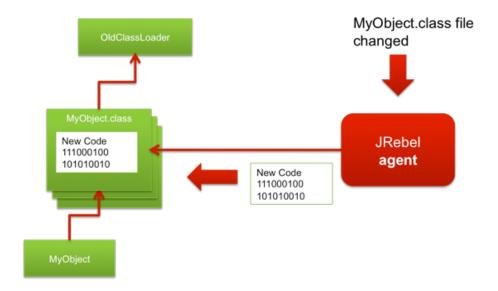
Importantly, when loading updates to a class, JRebel preserves all of the existing instances of that class. This allows the application to continue working, but means that when adding a new instance field it will not be initialized into the existing instances, since the constructor will not be rerun. State is preserved!
