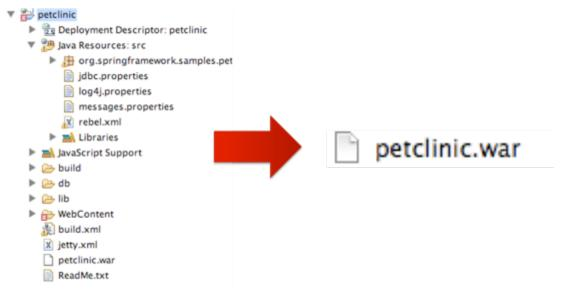
This allows for instant updates of not just classes, but any kind of resources like HTML, XML, JSP, CSS, .properties and so on. For Maven users, the JRebel Maven plugin will automatically generate the necessary rebel.xml file.
