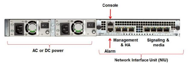
Plug the slot 0 port 0 (s0p0) interface into your outside (ATT next-hop facing) network and the slot 1 port 0 (s0p1) interface into your inside (CUCM server-facing) network. Once connected, you are ready to power on and perform the following steps.
