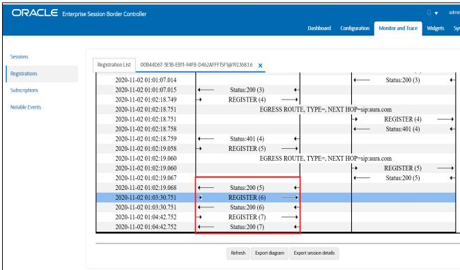
We can also make calls between these phones and we can verify the signaling path. The above call is made from access side to core side.
