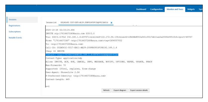
Similarly, we can also make calls from core side to access side and check the SIP path. Here the call is converted to TLS after reaching SBC.
