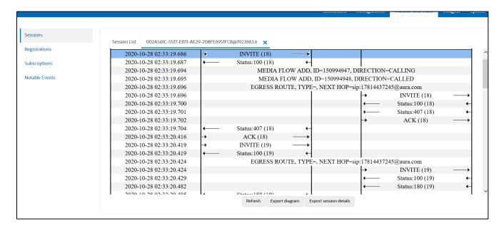
Here the INVITE from access side comes with TLS protocol and from SBC it is changed to TCP/UDP
