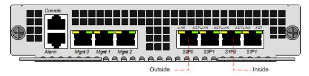
Plug the slot 0 port 0 (s0p0) interface into your outside (subscribers facing) network and the slot 0 port 1 (s1p0) interface into your inside IMS network. Once connected, you are ready to power on and perform the following steps.
