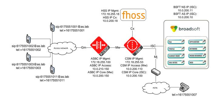
P-CSCF/SBC, CSM and Broadworks represent the Service provider domain infrastructure which provides PSTN service as well. Access network represent the different access technologies (DSL, UMTS, WLAN, etc) of subscribers and enterprises.
