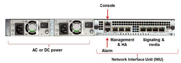
Plug the slot 0 port 0 (s0p0) interface into your outside (Bell Canada next-hop facing) network and the slot 1 port 1 (s1p1) interface into your inside (CUCM server-facing) network. Once connected, you are ready to power on and perform the following steps.
