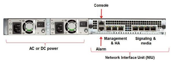
Plug the slot 0 port 0 (s0p0) interface into your outside (Telus next-hop facing) network and the slot 1 port 0 (s1p0) interface into your inside (CUCM server-facing) network. Once connected, you are ready to power on and perform the following steps.
