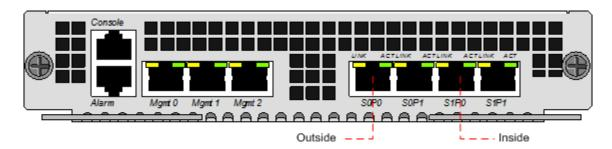
Plug the slot 0 port 0 (s0p0) interface into your outside (gateway facing) network and the slot 1 port 0 (s1p0) interface into your inside (mediation server-facing) network. Once connected, perform you are ready to power on and perform the following steps.
