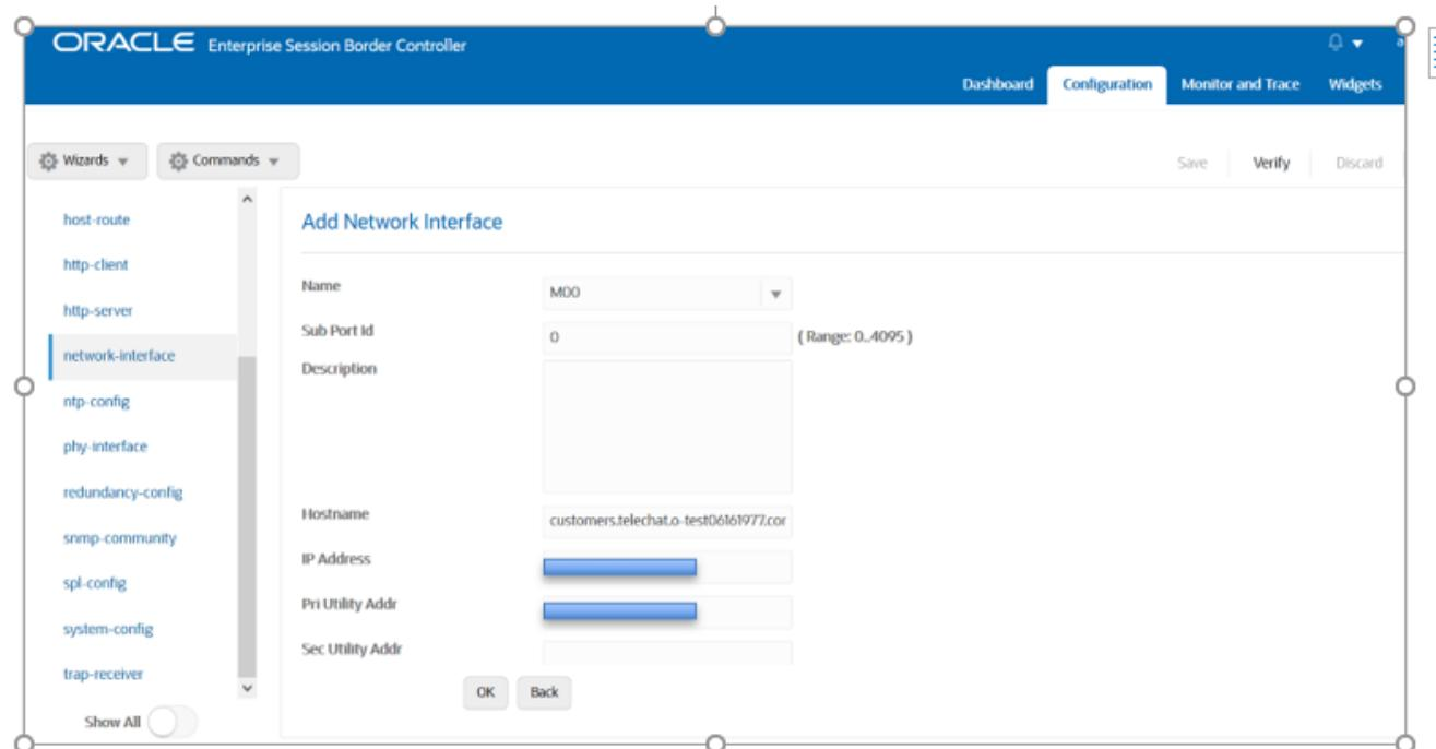
The screenshot shows the Oracle Enterprise Session Border Controller (ESBC) Configuration interface. The left sidebar has a tree view with options like host-route, http-client, http-server, network-interface (which is selected and highlighted in blue), ntp-config, phy-interface, redundancy-config, snmp-community, spl-config, system-config, and trap-receiver. The main panel is titled 'Add Network Interface' and contains the following fields:
