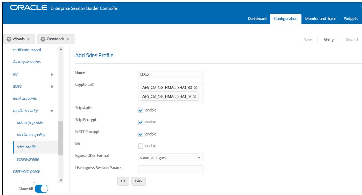
The screenshot shows the Oracle Enterprise Session Border Controller (ESBC) Configuration interface. The left sidebar shows a tree structure with nodes like certificate-record, factory-accounts, ike, ipsec, local-accounts, media-security (which is expanded to show dtls-srtp-profile, media-sec-policy, sdes-profile, sipura-profile, and password-policy), and a 'Show All' toggle. The main panel is titled 'Add Sdes Profile' and contains the following fields:
