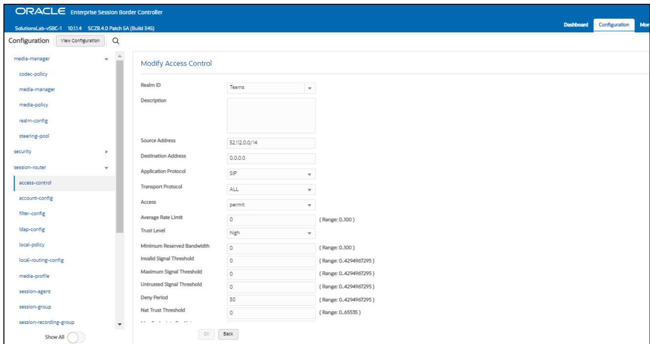
Notice the trust level on this ACL is set to high. When the trust level on an ACL is set to the same value of as the access control trust level of its associated realm, this creates an implicit deny, so only traffic from IP addresses configured as ACL's with the same trust level will be allowed to send traffic to the SBC. For more information about trust level on ACL's and Realms, please see the [SBC Security Guide, Page 3-10](#).
