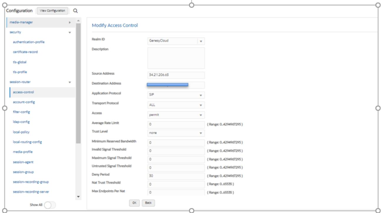
Similarly create ACL entries for each Microsoft Teams IP Addresses as shown in the below example. Microsoft Teams has two subnets, 52.112.0.0/14 and 52.120.0.0/14 that must be allowed to send traffic to the SBC. Both must be configured as an access control on the Oracle SBC and associated with the realm facing Teams. Use this example to create ACL's for all MSFT Teams subnets. This example can be followed for any of the public facing interfaces, ie...SipTrunk, etc...
