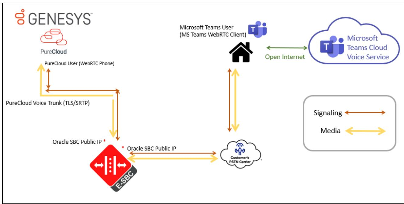
Above figure illustrates the connection between Genesys Cloud Cx, Oracle SBC and Microsoft Teams Direct Routing. Both Cloud Cx and Microsoft Teams are connected to the Oracle SBC Public FQDN /IP
