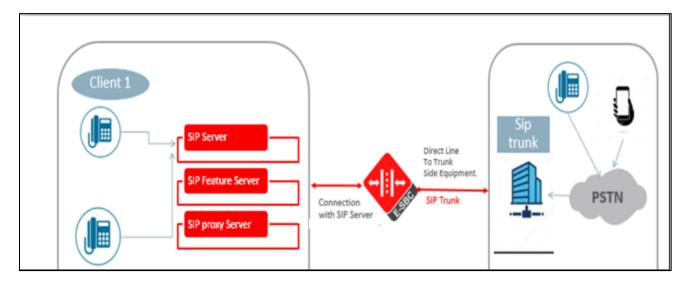
The lab setup used for the testing is given below specific to Genesys Pure Engage with Twilio SIP trunk.
