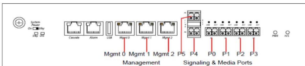
Plug the slot 0 port 0 (s0p0) interface into your inside (SFB server facing) network and the slot 0 port 1 (s0p1) interface into your outside (gateway facing) network. Once connected, perform you are ready to power on and perform the following steps.
