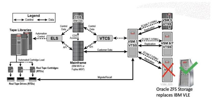
"Oracle ZFS Storage as an IBM mainframe backup/archive through Oracle's StorageTek VSM" use case depicts VMS7 VTSS supporting emulated tape connectivity to IBM MVS hosts and attachment to Real Tape Drives (RTDs), Virtual Library Extensions (VLEs), and other VTSSs to provide virtual tape device emulation, virtual tape cartridge images, and additional buffer capacity for the IBM MVS environment.
