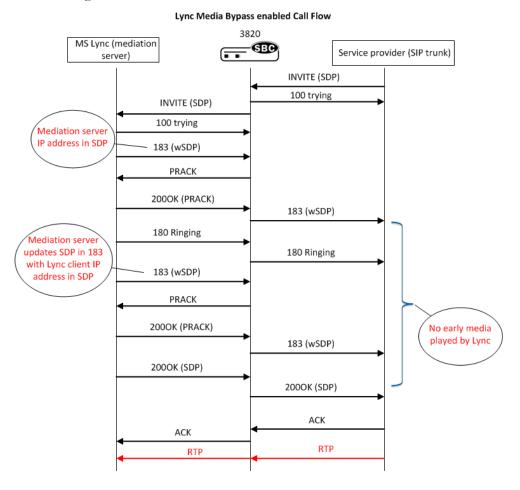
**Note:** that after signaling 183 with SDP, Lync never plays any early media and expects gateway (E-SBD) to signal appropriately to the SIP Trunk provider to follow RFC 3960 and play local RBT. The second 183w SDP coming from Mediation server which is forwarded to the SIP trunk and stops the local RBT which was started after 180 Ringing was sent; hence PSTN caller would hear a silence before Lync client answers call.
