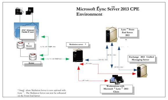
The Lync server Mediation server and the Acme Packet series SBC are the edge components that form the boundary of the SIP trunk. This document describes the configuration of the Lync server and the SBC and the results of the test plan.
