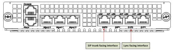
Plug the slot 0 port 0 (s0p0) interface into your SIP trunk provider (SIP trunk facing) network and the slot 0 port 1 (s1p0) interface into your Lync (Lync mediation server-facing) network as shown in the diagram above. Once connected, you are ready to power on and perform the following steps.
