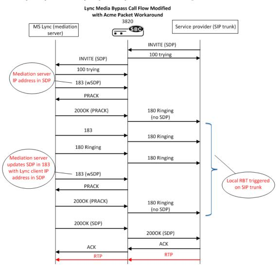
The following header rules needs to be included in the manipulation that is applied on the realm or sip-interface facing Lync to modify the signaling traffic sent from Lync.
