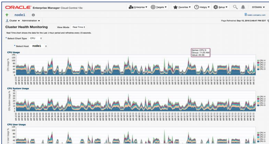
Figure 5: CPU utilization metric broken down further into CPU usage, CPU system usage, and CPU user usage in Cluster Health Monitor
