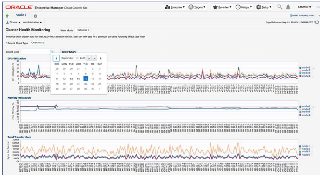
Figure 4: Historical review of metrics collected by Cluster Health Monitor for multiple nodes in the cluster as seen in Enterprise Manager
