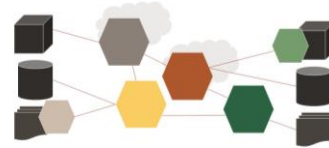
Figure 7: Conceptual topology difference between a Hub and a Mesh
