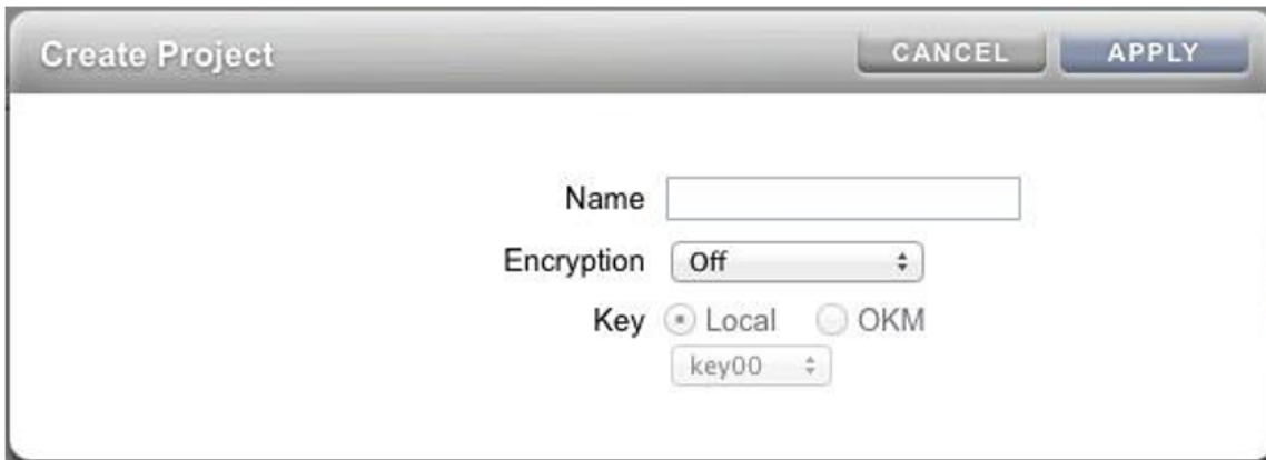
Figure 18. Encryption toggle in the Create Project dialog window of Oracle ZFS Storage Appliance
