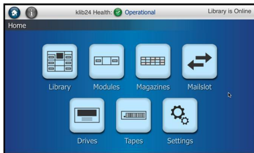
Figure 1. StorageTek SL150 modular tape library touchscreen operator panel
