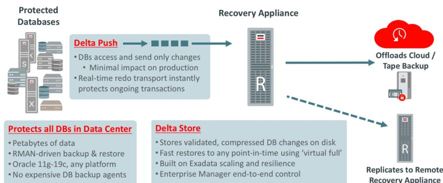
Figure 1. Zero Data Loss Recovery Appliance: Architecture Overview
