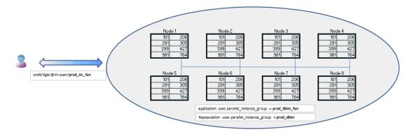
This shows clients connecting with the "prod\_im\_fan" service that is managed so that a failed instance is disabled from the service.
