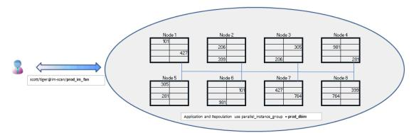
This shows clients connecting with the "prod\_im\_fan" service that is managed so that a failed instance is disabled from the service. The application uses the "prod\_dbim" service for parallel\_instance\_group parameter.
