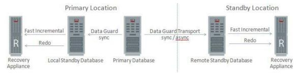
Figure 7: Multi-Standby Configuration with Local HA Failover
