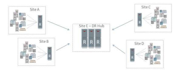
Figure 4: Hub and Spoke Architecture Using Recovery Appliance Replication
