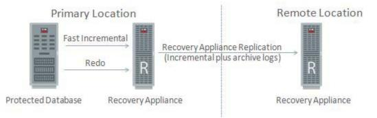
Figure 3: Recovery Appliance and Silver Reference Architecture
