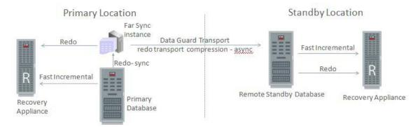
Figure 6: Zero Data Loss Failover at Any Distance Using Active Data Guard Far Sync
