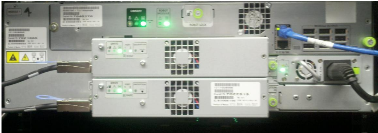
Figure 2: Rear of Oracle StorageTek SL150 tape library with two LTO SAS attached tape drives.
