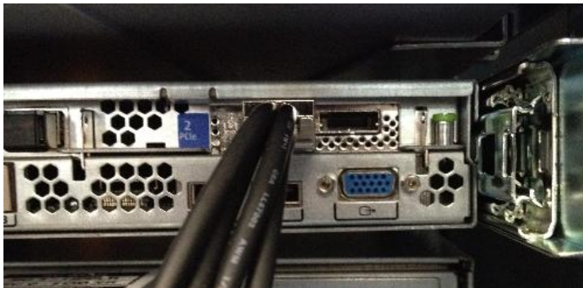
Figure 3: Rear of Oracle's Sun Server X3-2 with multi-pronged SAS cable connected to SAS HBA card.
