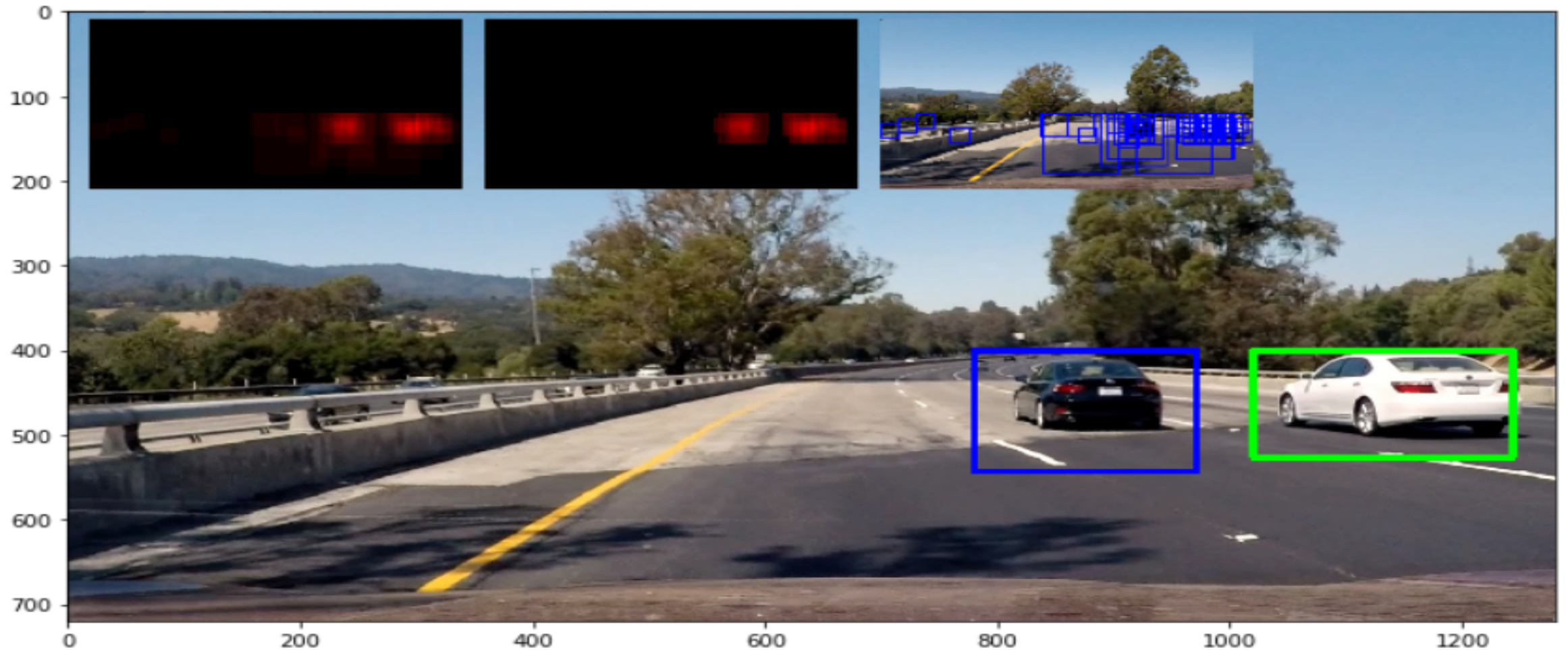
Detected vehicles with heatmaps and thresholding
