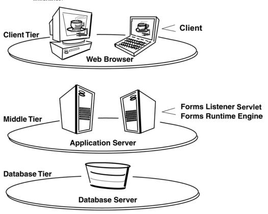
Figure 15–2 Forms Services Web-based architecture
