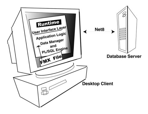
Figure 15–1 Legacy Forms Server client-server-based architecture
