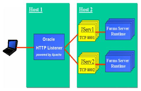
Figure 4. Multiple JServ engines on multiple hosts
