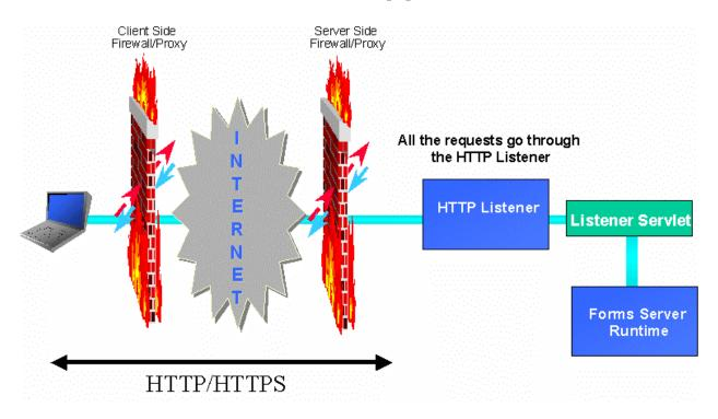
Figure 2. New architecture using the Forms Listener Servlet
