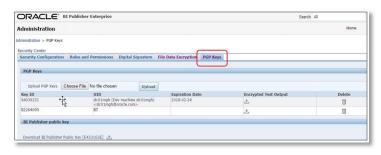
PGP Encryption of reports during FTP delivery has been there as a feature; however there were manual steps to request and to apply the PGP Keys in the environment. Now Administrators can upload and manage PGP Keys from the Administration page and the Filter Command is automatically populated on selection of the PGP key. Therefore, FTP delivery encryption is now a self service feature and a matter of just few clicks.
