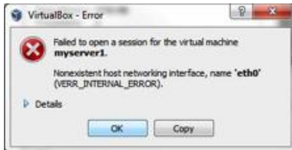
Figure 13: Probable network error when attempting to start a virtual machine for the first time
