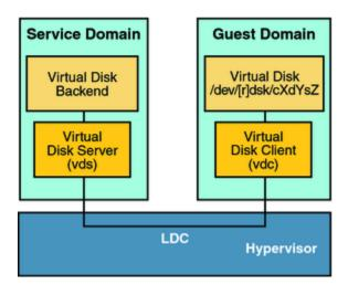
Figure 3 Virtual Disks with Oracle VM Server for SPARC
