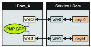
Figure 1 Two Virtual Networks Connected to Separate Virtual Switch Instances
