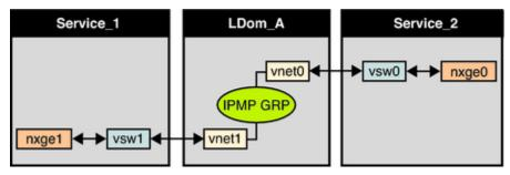
Figure 2 Virtual Network Devices Each Connected to Different Service Domains
