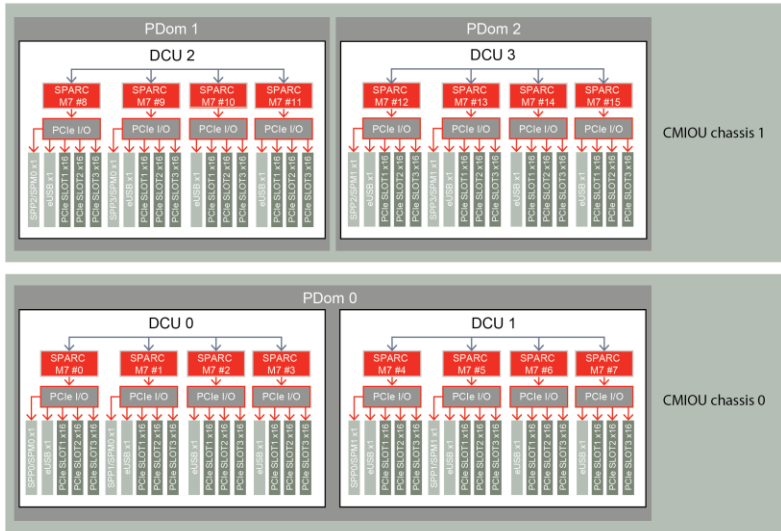
Figure 3. The SPARC M7-16 server can be flexibly configured with one, two, three, or four PDom (three PDom shown), each with two SPPs for active/passive failover.
