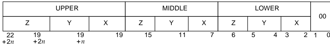
FIGURE 7-5 Three Dimensional Array Blocked-Address Format (ARRAY32)
