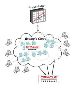
TimesTen In-Memory Cache Grid was configured on all 8 compute nodes in the Exalogic machine. Four cache grid members were configured for each compute node to take advantage of the compute power and available RAM.
