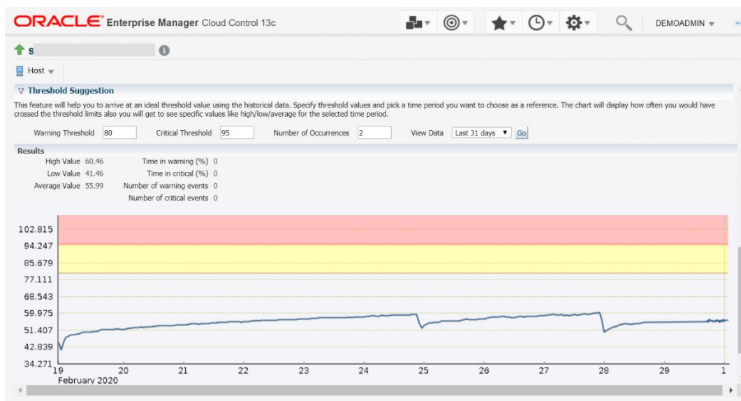
Figure 30. The threshold suggestion region shows you the value of the metric over a recent period of time.
