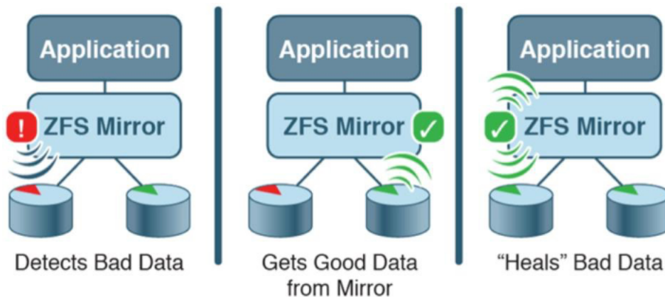
Figure 5. Example of how ZFS self-healing architecture corrects a corrupted block.
