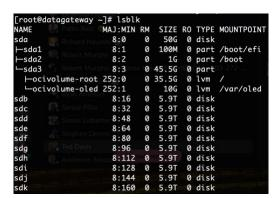
Figure 2. Attached block devices to the Oracle Linux Data Transfer Gateway instance
