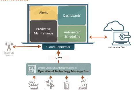
**Figure 2** Oracle IoT Intelligent Applications architecture for energy and water companies
