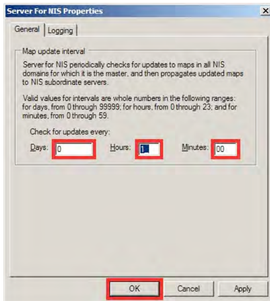
Figure 45. Setting propagation frequency for map updates in Server for NIS Properties window
