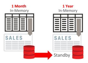
Figure 4. Example of how the IM column store on the standby database can have very different content to the primary.
