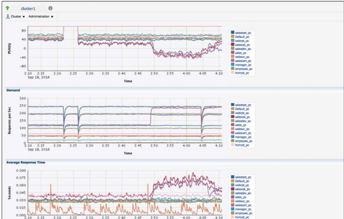
Figure 14: Quality of Service Management display of the performance history of the workloads
