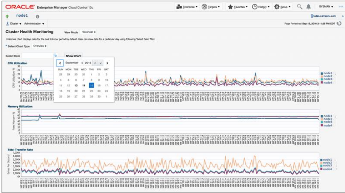
Figure 4: Historical review of metrics collected by Cluster Health Monitor for multiple nodes in cluster as seen in Enterprise Manager
