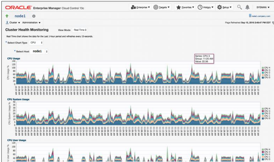
Figure 5: CPU utilization metric broken down further into CPU usage, CPU system usage, and CPU user usage in Cluster Health Monitor
