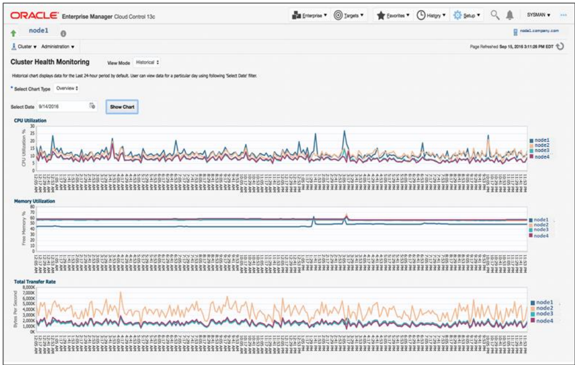
Figure 3: Metrics collected by Cluster Health Monitor for multiple nodes in cluster as seen in Enterprise Manager
