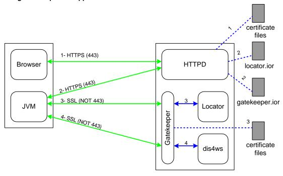
The Locator and Discoverer Sessions objects (dis4ws processes) only use IIOP, they do not support SSL encryption. To secure communication between the Plus client and the Oracle9iAS middle-tier we once again turn to the Gatekeeper:
