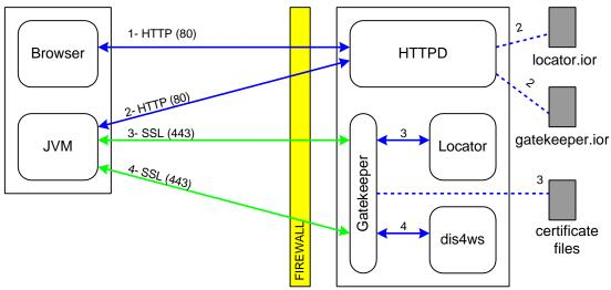
The diagram above is almost identical to section 3.3.2. The differences are the inclusion of a firewall and configuring the HTTP server to listen to port 80 without SSL.
