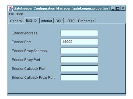
On the Exterior tab, specify the port number in the Exterior Port field. The Gatekeeper will listen for both IIOP and HTTP traffic on that port.
