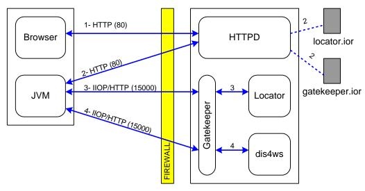
A firewall administrator  $\underline{is}$  likely to open the firewall for traffic to a specific port on the Oracle9iAS machine. As stated above, the problem is that IIOP does not restrict the TCP port used for connections. The Gatekeeper resolves this problem:
