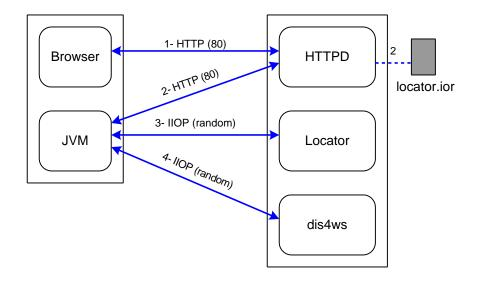
The Discoverer 4i Plus client is a Java applet. The diagram above shows how Plus is launched and subsequently communicates with the Oracle9iAS middle-tier.
