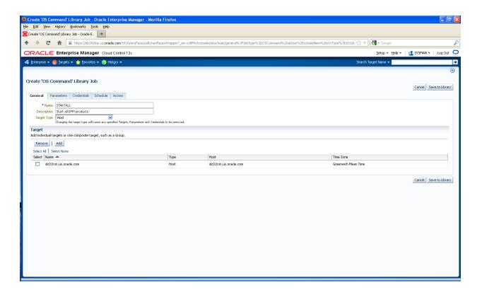
5. Click the "Parameters" tab and provide the full path for the script to be invoked. Specify any additional parameters needed as well.
