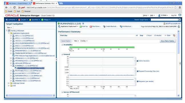
Similarly, operations, log messages and metrics can be accessed at the Domain, Server, and Application Deployment levels for EPM System products by navigating to the appropriate targets in these pages. The WebLogic Administration Server must be running for some operations such as Log Viewing, Server Start Up and Shut Down, and so on.
