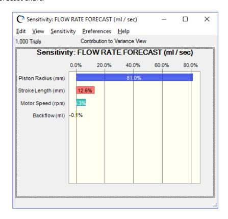
The Piston Radius contributes 81.0% of the variance in the Flow Rate forecast, so this is the next logical place to improve the design. Once you have addressed this parameter, you can re-run the simulation and view the new – and hopefully improved – capability metrics.
