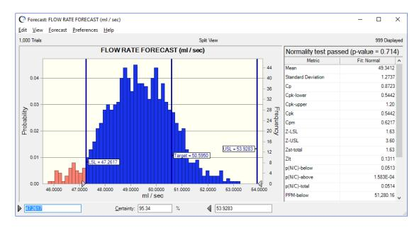
Crystal Ball automatically sets marker lines at each parameter and positions the triangular grabbers at the spec limits, which are 47.2617 and 53.9283 ml/sec. The certainty that the flow rate will be within the required limits is 95.34%.
