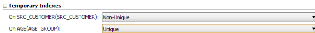
Figure 15 – Two temporary Indexes (Non-Unique and Unique) will be created for optimizing the execution of the join between SRC_CUSTOMER and AGE_GROUP.
