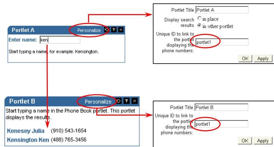
Figure 5 – Wiring Portlets Through Personalization
