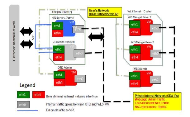
The green and red are representing two external user defined network interfaces. The gray represents to internal traffic going between OTD and WebLogic VMs. The blue represents to the external traffic to OTD VIP.
