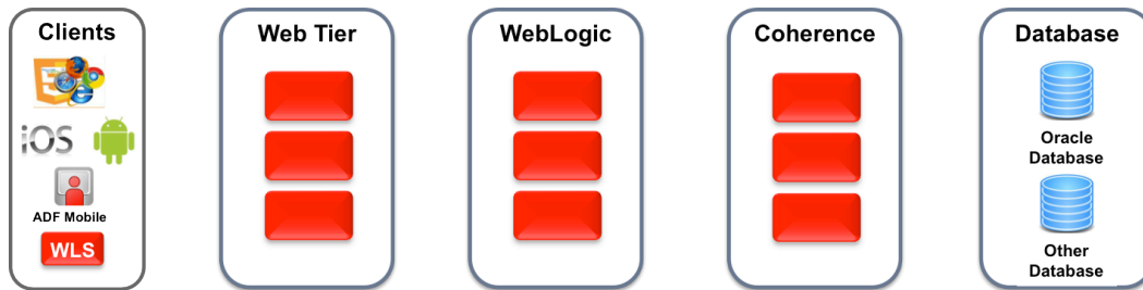
Figure 1: Typical Oracle WebLogic Suite Production Deployment Topology
