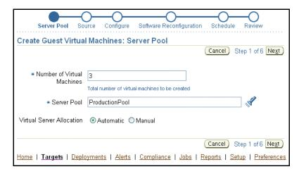
Figure 5. Oracle Enterprise Manager provides a simple, flexible approach to provisioning guest virtual machines. New guest virtual machines can be created using ISO images of operating systems, Oracle VM Templates, and PXE bootable guest virtual machines that boot from the network.
