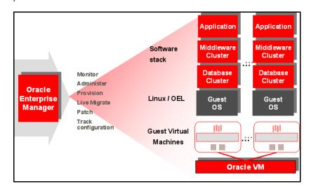
Figure 1. Oracle VM Management Pack enables a comprehensive view of the software stack to optimize the allocation of server resources from the top down.
