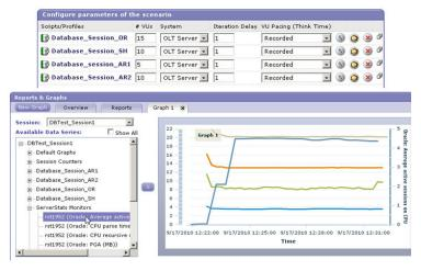
Figure2. Oracle Load Testing allows you to scale up the test scripts against any number of concurrent virtual users to analyze database performance under load.
