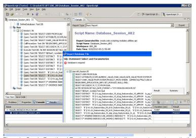
Figure 1. Oracle Functional Testing's OpenScript allows you to create synthetic database test scripts to test your Oracle Database. Database transactions can be automatically imported from Database Replay workload captures from your production database
