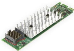
Figure 18. The Sun Dual 10 GbE PCIe 2.0 FEM provides two 10 GbE interfaces.
