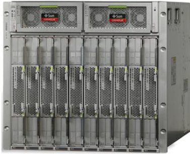
Figure 1. The Sun Netra 6000 AC chassis provides two power supply units (PSUs) and supports up to 10 Sun Netra 6000 server modules in 10U.
