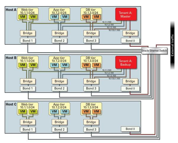
Figure 4: Virtual Network Services deployed with Oracle Ethernet Switch ES2-64 or ES2-72
