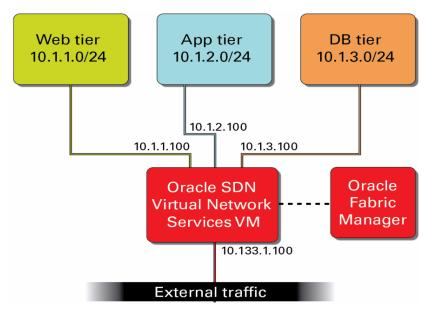
Figure 2: Virtual Network Services in a three-tier architecture for a tenant
