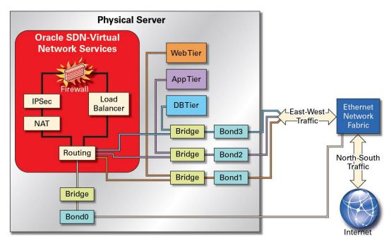
Figure 3: Virtual Network Services deployed per tenant
