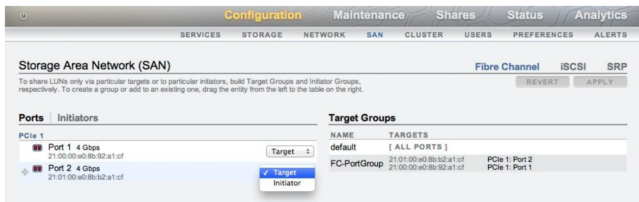
Figure 2. Setting a PCIe port to target mode in the Oracle ZFS Storage Appliance
