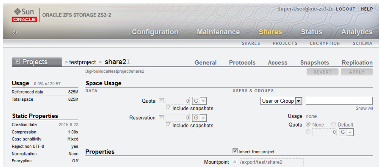
Figure 4. Determining the ZFS path of a share using the Oracle ZFS Storage Appliance BUI
